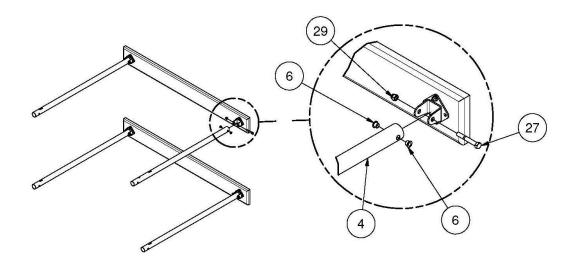
Install the outer pipe weldments to the hinge points on the lower two wood pads. Install the bushings (Item 6) into both sides of the pipe before installing the pipe into the hinge bracket.
