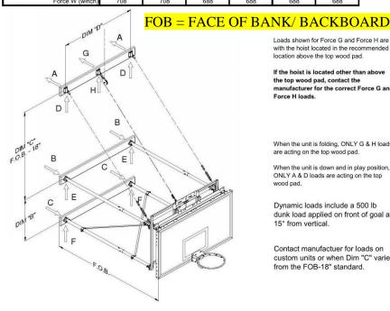
Loads shown for Force G and Force H are with the hoist located in the recommended location above the top wood pad.
