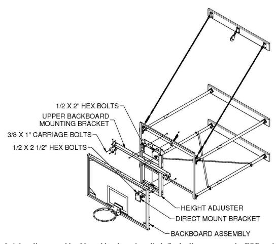
Once the height adjuster and backboard has been installed, final adjustments to the FOB and chain tension can be made.
