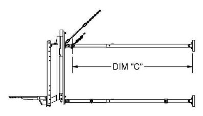
Slide the pull up tube on the upper extension arms until the center of the tube is Dim "C" from the upper wood pad. Make sure the tube is parallel with the face of the backboard.
