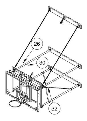
The final step of the assembly is to level the frame extension arm by adjusting the chain tension with the turnbuckles. It is important to not over adjust the chains as this causes undue stress on the chain anchor points. Chain tension should be no more than enough to level the side frame tubes.
