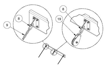
Install the #5 pulley onto the center bracket of the top wood pad using the 5/16" quick link. Make certain link is fully closed and tightened.
