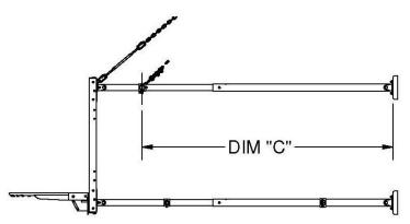
Slide the pull up tube on the upper extension arms until the center of the tube is Dim "C" from the upper wood pad.
