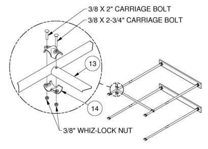
Install the pull up cross tube (Item 13) onto the top extension tubes.
