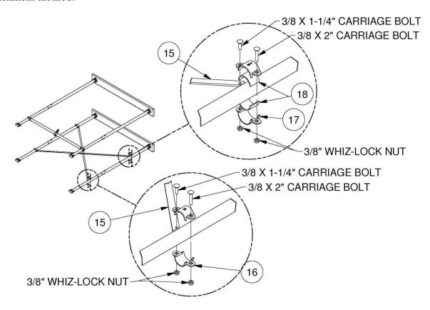
**Note:** the 3/8 x 2", 3/8 x 1-1/4" carriage bolts, and the 3/8" whiz-lock nuts are supplied with item 16 and are not listed in the parts list. DO NOT fully tighten these clamp bolts at this time as it may be necessary to reposition them after the board and goal are installed and the FOB is set.
